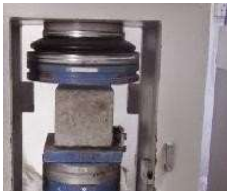
Fig.3: Testing on UTM.
